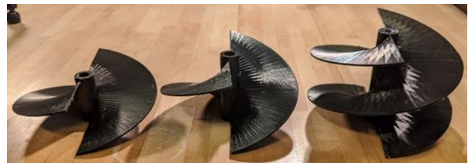
Figure 5.1: 3D printed rotors used in scale model testing
