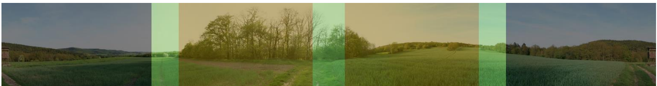
Figure 8.5: Pilot point-of-view FOV, 18% is unobstructed, cameras increase pilot FOV by over 500%
