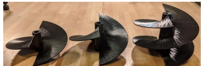
Diameter = 150mm Diameter = 150mm Diameter = 150mm \sigma = 1 \sigma = 1 \sigma = 2 Height = 50mm Height = 75mm Height = 100mm \theta_{root} = 57.8^\circ \theta_{root} = 67.3^\circ \theta_{root} = 57.8^\circ \theta_{tip} = 12.0^\circ \theta_{tip} = 17.7^\circ \theta_{tip} = 12.0^\circ
