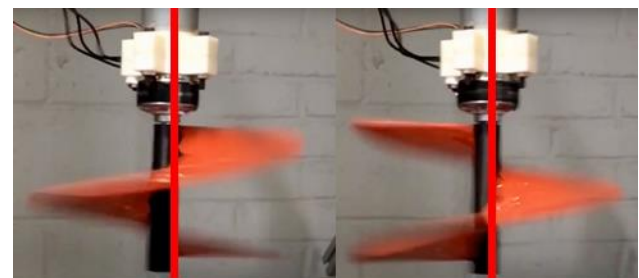
Figure 4.17: Still images from a video showing inherent vibrations of a Single-Turn Aerial Screw
