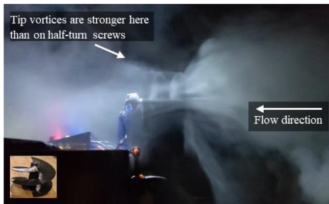
Figure 4.26: Flow Visualization for Double-Turn, Single Surface, Concentric Aerial Screw Aerial Screw, \theta_{root} = 57.8^\circ
