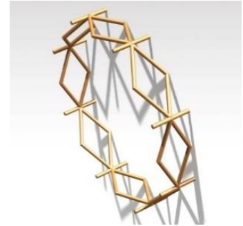
Figure 6.14: Diamond bay cross section
