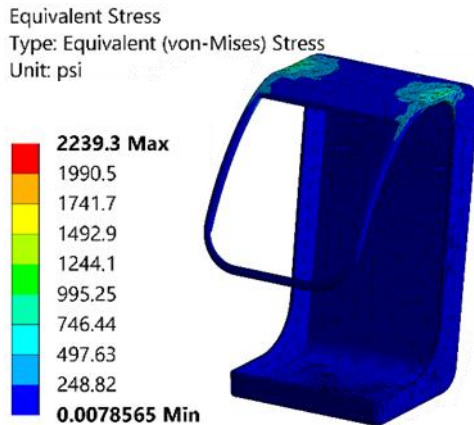
Figure 6.20: Cockpit stress response
